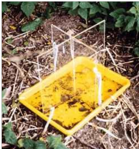
Fig. 2 Window-trap in yellow pan-trap.
